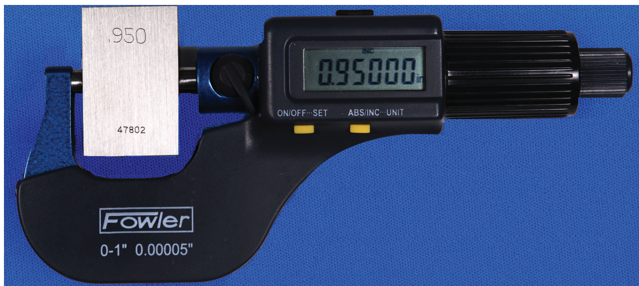
Figure 3.21 A modern digital micrometer capable of measuring in both inches and millimeters. A NIST-traceable gauge block standard is being used to test the accuracy of the micrometer.
