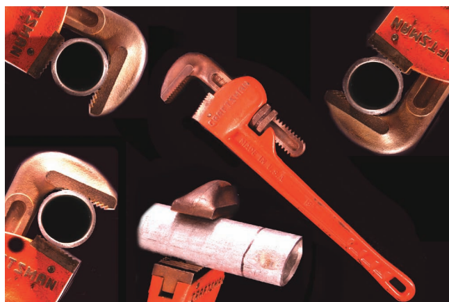
Figure 9.62 Application of a pipe wrench to an iron gas pipe.
