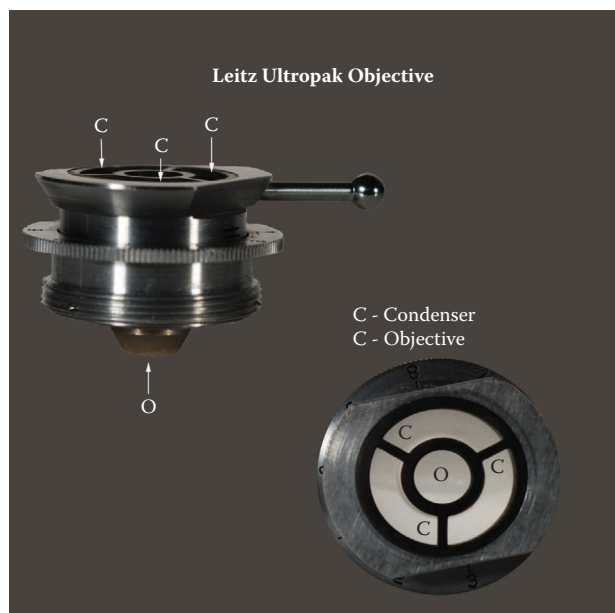
Figure 2.13 Low power Leitz® Ultropak objective lens. The outer ring of lens sections (C) surrounding a central objective lens (O), act as a condenser, condensing the light coming from an attached illuminator. The center lens objective O collects the reflected light that illuminated the specimen and forms an image of the specimen. This method of illumination will be discussed in more detail in another portion of this chapter.
