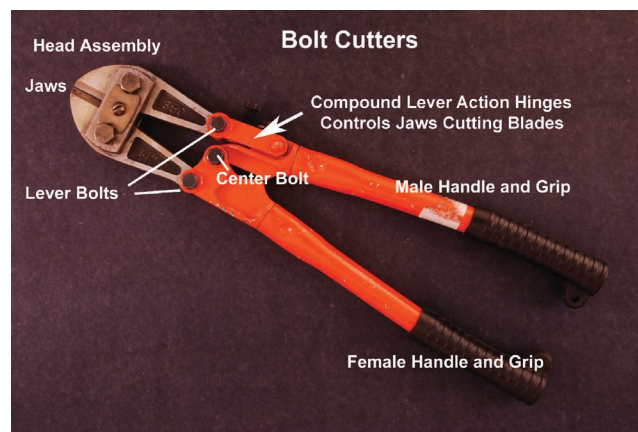
Figure 9.94 A common type of bolt cutter and its parts.
