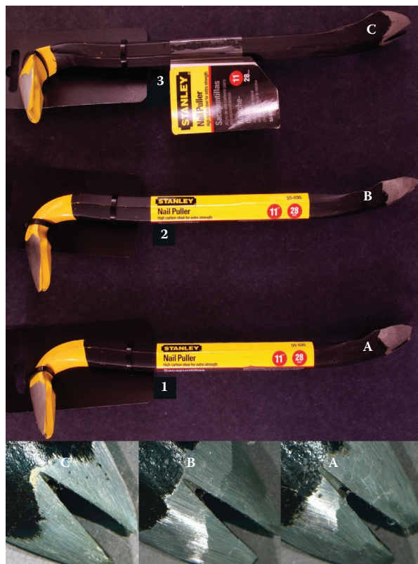
Figure 9.18 Three nail pullers. Note the obvious difference in the finish of designated claws due to the finishing process (grinding). All six claws on these tools have different shapes and striation patterns.
