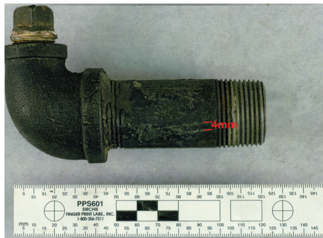
Figure 7.6 Opposite side of pipe in Figure 7.3. Spacing between teeth toolmarks on the pipe is 4 mm.
