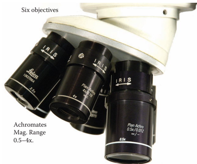
Figure 2.18 A set of Leica plan achromatic objective lenses. Each has a fixed NA, a fixed magnification and a built in iris diaphragm. The range of magnification with a 10× eyepiece is 5.0 to 40×. The author prefers the use of fixed magnification objective lenses over the zoom type lens.
