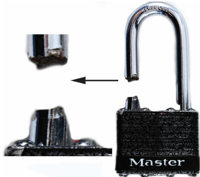
Figure 4 The morphology of the cut marks present on the end of the lock's shackle indicates that a shearing type bolt cutter was used to cut the shackle.
