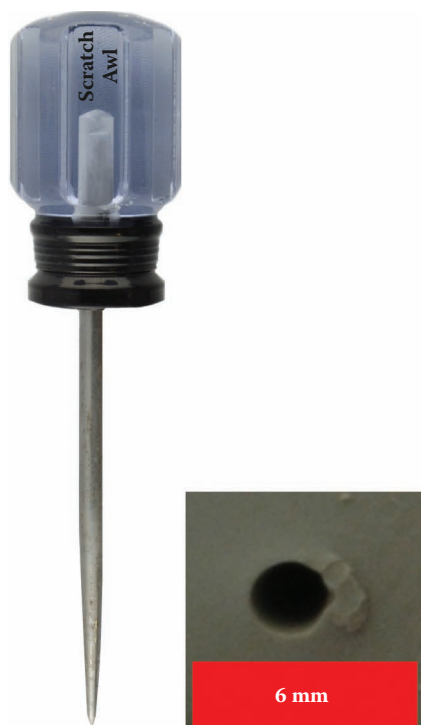
Figure 9.8 An awl for punching holes. Awls produce toolmarks that are very similar to ice pick marks.
