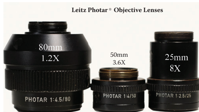
Figure 2.15 Three Leitz Photar® macro lenses provided with RMS screw tread for use in photomicrography and with comparison microscopy. The range of magnification of these three lenses is ideal for use in toolmark comparisons.
