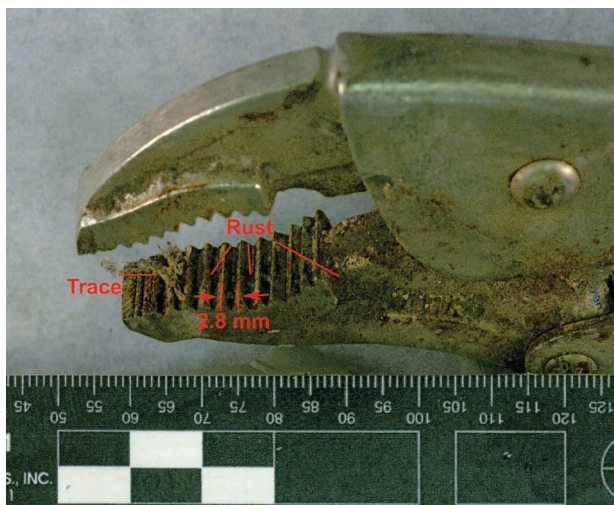
Figure 7.4 Vise-grip with undisturbed traces of old twine and undisturbed deposits of rust on the serrated teeth of the lower jaw.
