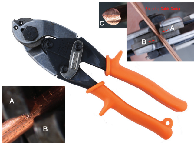
Figure 9.97 The shearing cutting action of a cable cutter blade (A) pushes the metal in one direction while blade B pushes the metal in the opposite direction until the cable fatigues (C).
