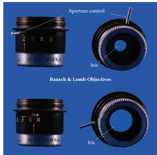
Figure 2.12 Old style objectives produced by an early manufacturer of comparison microscopes. The lens has a magnification of 2.5× and an NA of 0.08. The aperture numbers seen on this objective do not follow the convention associated with f -stops. In this instance the smaller number has a smaller aperture, while the larger number has a larger aperture.
