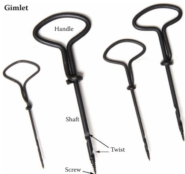
Figure 9.145 Various size gimlets are used to make small holes in wood.
