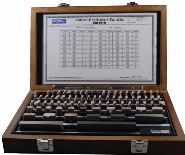
Figure 3.4 A calibrated set of NIST-traceable gauge blocks with certificate. Each gauge block is serial numbered and has its calibrated value marked on its front surface.
