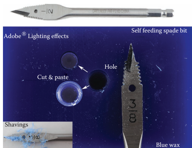
Figure 9.126 Self-taping spade bit with standards in wax. Adobe lighting effects in render menu used to look down into hole.
