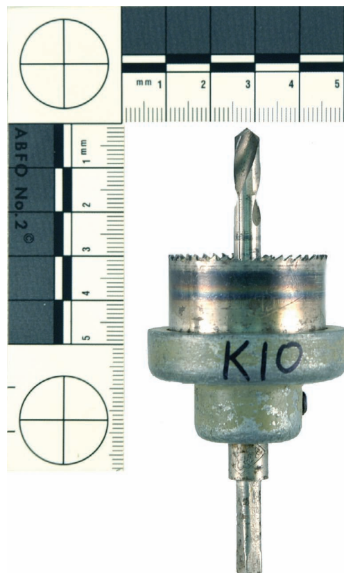
Figure 9.132 Hole saw. Used for cutting holes in doors for lock cylinders and/or door knob apparatus.
