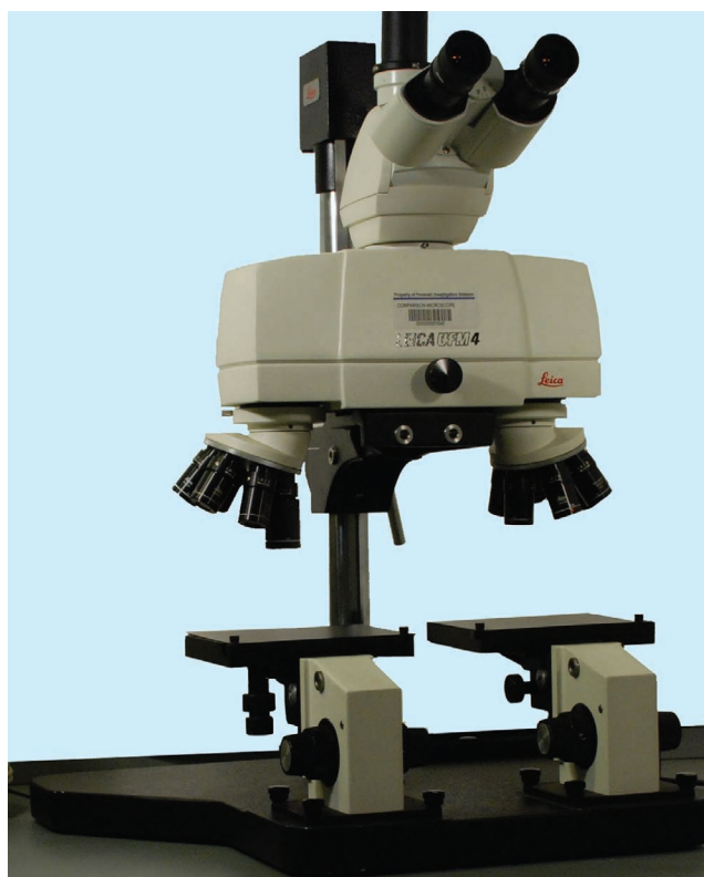
Figure 2.42 A modern 21st century Leica® comparison microscope outfitted with 2 sets of 0.5×, 1.0×, 1.5×, 2.0×, 2.5× and 4.0× objectives of matching 10× eyepieces. Additional objective lenses are available (i.e., lower power plan apochromates).
