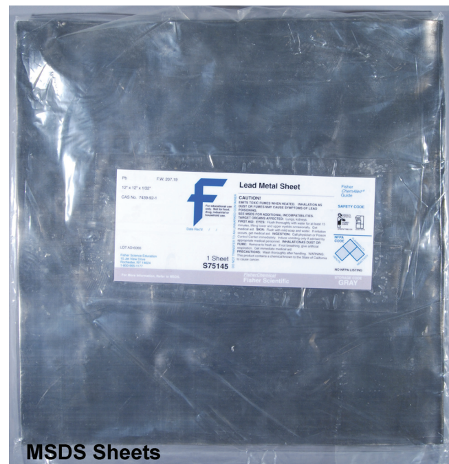
Figure 6.8 Pliable lead sheets 12 × 12 in. square, and \frac{1}{32} in. thick are available commercially and should be supplied with a materials safety data sheet (MSDS).
