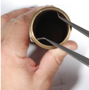
Figure 3.11 The tilted position of the shown caliper will result in an incorrect assessment of the workpiece's diameter.
