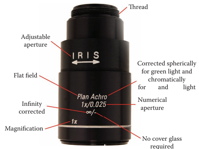
Figure 2.19 Above is shown a Leica® plan achromatic, fixed magnification, fixed NA objective lens.
