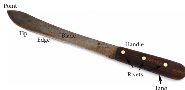
Figure 9.103 A typical kitchen knife and its major components.
