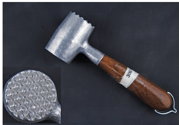
Figure 9.52 (a) Four different types of mallets. (b) Meat mallet made of aluminum.
