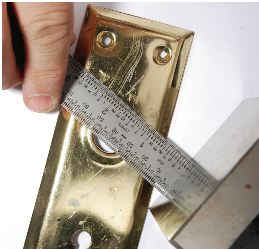
Figure 3.28 The width of the major toolmark present on the door lock plate is being measured directly with a steel rule and a right angle block.
