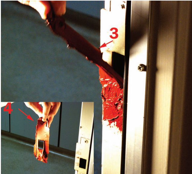
Figure 5.16 (3) Remove the entire cast from the subject area and photograph the removed cast.
