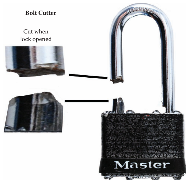
Figure 9.96 A staged burglary in which the lock's shackle was cut while opened with a shearing action bolt cutter.
