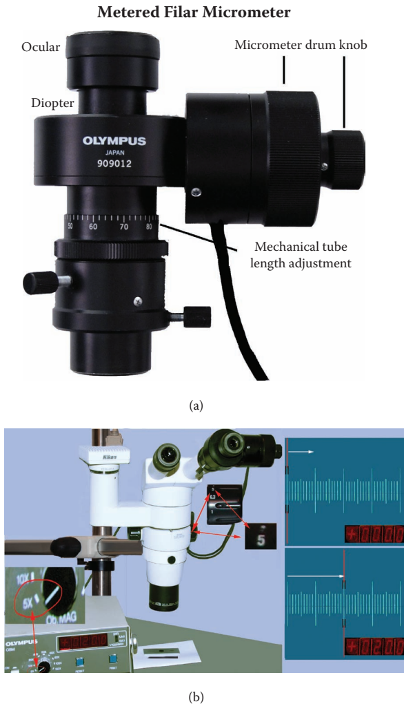
Figure 4.13 (a) A Filar micrometer attached to an electronic, digital metering system. (b) A calibration check of a digital Filar micrometer set at the 5× metering position, with the microscope set to the 5 zoom position. The movable line set in this diagram is colored red for demonstration purposes; normally, it is black. First, set the units of measurement being utilized (inches). Next, set the desired zoom knob position (5), and then focus the microscope until a sharp image of the stage micrometer is obtained. Next, align the movable line set of the Filar micrometer with the first division on the stage micrometer. The meter should now read +000.0. Then, rotate the micrometer's drum knob; this action will cause the movable line set to travel from left to right. Next, stop at the desired stage micrometer division and take a meter reading. In the above example the movable line set traversed twenty stage micrometer divisions, or twenty thousandths of an inch, the exact value covered on the stage micrometer and recorded on the meter.
