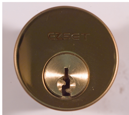
Figure 7.27 Questioned lock cylinder received for examination showing no signs of tampering or damage.
