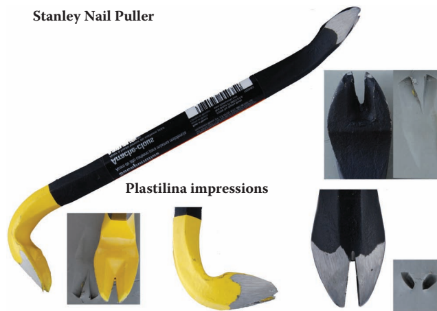
Figure 9.17 Nail puller with the resultant toolmarks.
