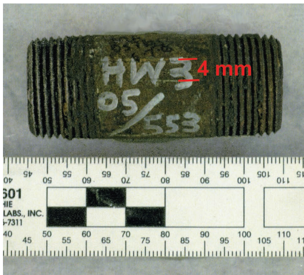
Figure 7.2 Pipe with toolmarks. The spacing between toolmarks on the pipe is 4 mm.
