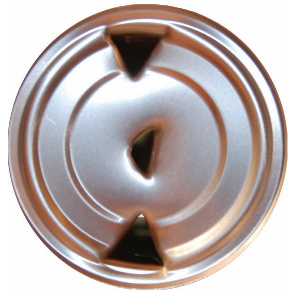
Figure 5 The pattern or overall morphology (class characteristic pattern) of the puncture marks on this can's top instantly tells one that a beer can type can opener is responsible for the holes.
