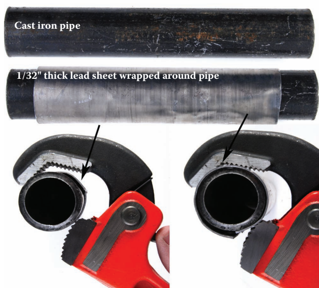
Figure 9.65 A pipe wrench's tooth marks being prepared on a sheet of \frac{1}{32} in. lead, wrapped around a 1\frac{1}{2} in. cast iron pipe. Note the movement of the teeth (left to right) within the jaws when pressure is applied to the handle.
