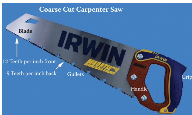
Figure 9.30 Coarse cut saw with twelve teeth per inch on the blade's front portion, and nine teeth per inch on the back portion of the 14 in. blade. Gullets are positioned for waste (sawdust) to escape.
