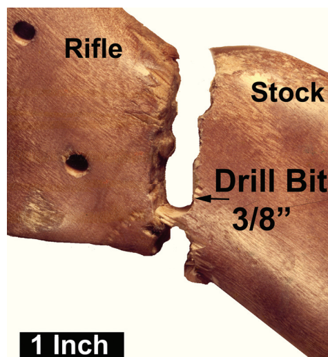
Figure 7.11 The two pieces of gun stock aligned, showing the space caused by a \frac{3}{8} in. drill bit.
