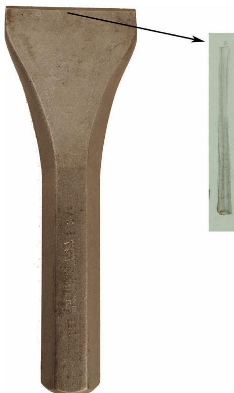
Figure 9.119 Mason's chisel used to break bricks, cinder blocks, and concrete.
